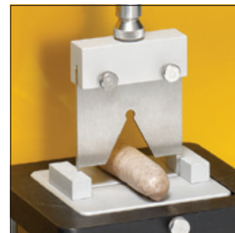
TA-SBA F Shear Blade for products where a cutting-shear test is meaningful: meat, fish, sausage, etc. Fixture Base Table required.
