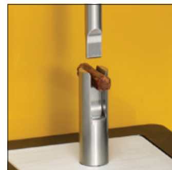
TA-VBJ F Volodkevich Bite Jaws for testing bite force of meat products using shear cutting-test. Fixture Base Table required.
