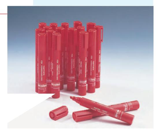
Attention: The test fluid of Ouicktest38 contains solvent. This might cause wrong results being displayed on materials or surface coatings not being solvent resistant!
